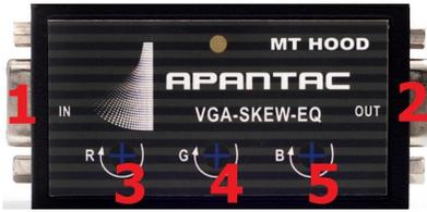
1. VGA port - connect to VGA-SKEW-EQ Cable
